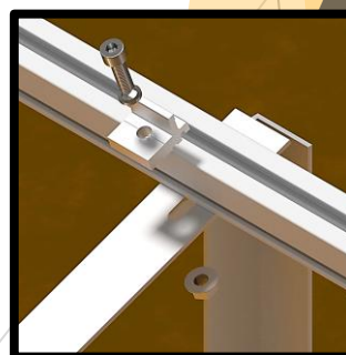
Rail connection to incline channel
